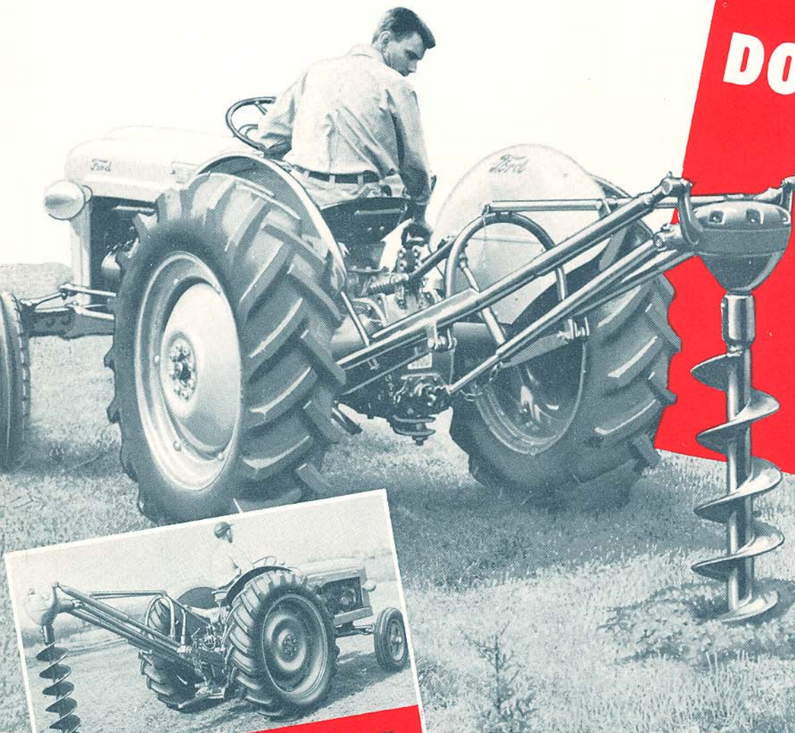
ON THE FORDSON MAJOR TRACTOR bigger, heavier jobs can be a "cinch" with a power-matched Danuser Post Hole Digger.
